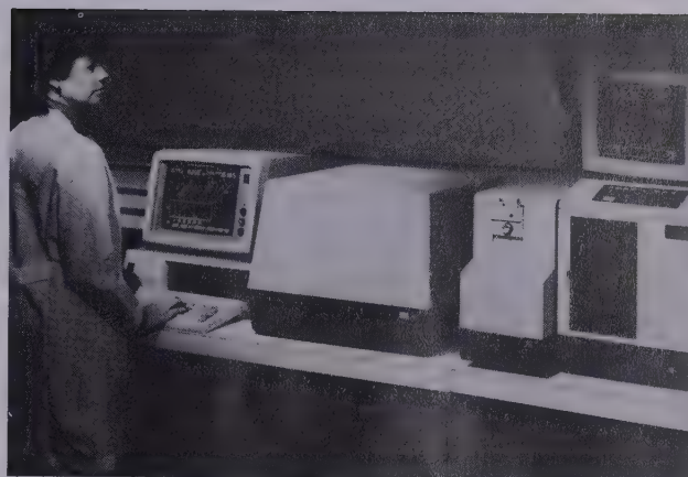
A gas chromatography apparatus (on the right) can be connected to a mass spectrometer (towards the left) with the output from each analysed by computer.
