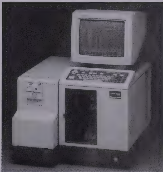
A sophisticated gas chromatography machine has its output directly analysed by computer.
