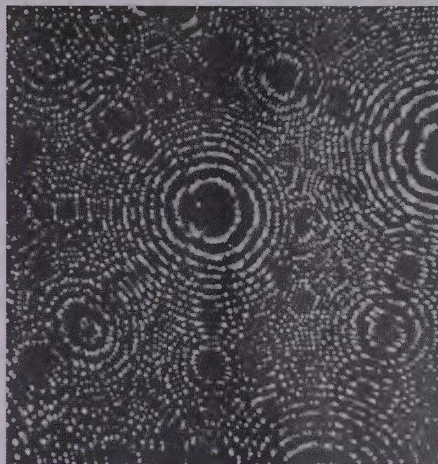
This is a field ionisation image of the surface of a nickel-molybdenum alloy, \text{Ni}_3\text{Mo} . Taken from Figure 9.5 of K. M. Bowkett & D. A. Smith, Field-Ion Microscopy , North-Holland Publishing Co., Amsterdam, 1970.
