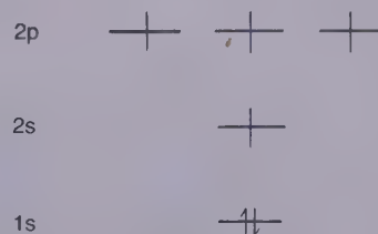
Figure 17.8 The electron structure for a carbon atom that has gained sufficient energy for one of its 2s electrons to enter the empty 2p orbital. There are now four unpaired electrons. (Note: as this is a hypothetical state of a carbon atom we cannot say what the orientations of the spins would be. For this reason the heads are left off the arrows)
