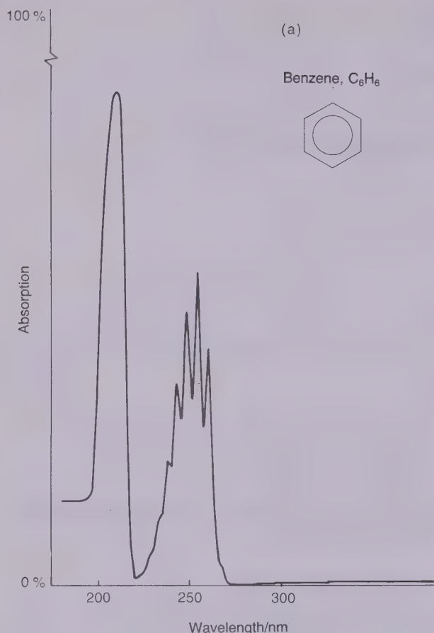
Figure 26.5 The ultraviolet absorption spectra of (a) benzene, in ethanol as a solvent, and (b) naphthalene, in methanol as a solvent
