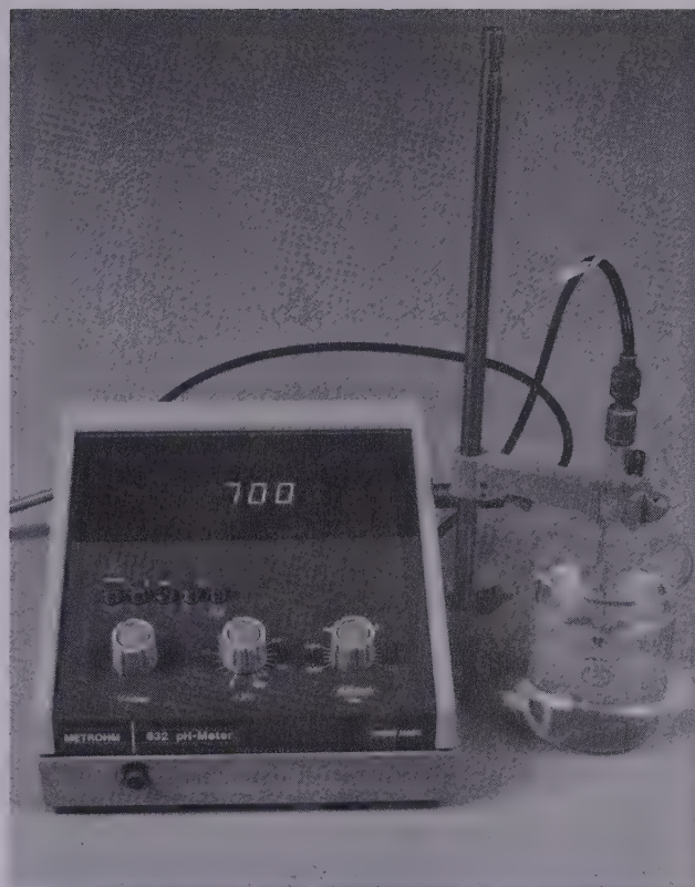
A typical pH meter and electrode.
