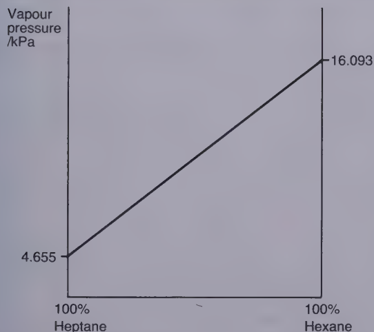
Figure 63.1 The vapour pressure–composition diagram for a mixture of hexane and heptane slopes in the opposite direction to the boiling point–composition diagram. (Low vapour pressure means high boiling point, and vice versa)
