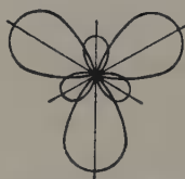
FIG. 54. Three sp^2 orbitals in the same plane but at angles of 120^\circ to each other.
