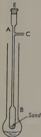
FIG. 8. Victor Meyer's apparatus for measuring vapour density.
