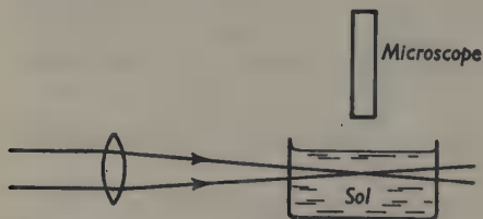
FIG. 164. Principle of the ultra-microscope.
